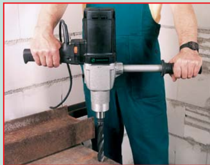
Up to 1 1/4" twist drill capacity
